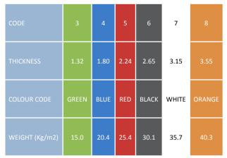
Although only milled lead manufactured to BS EN 12588 uses this thickness coding and colour system, it is always best to also refer to the British Standard when specifying sheet lead.
