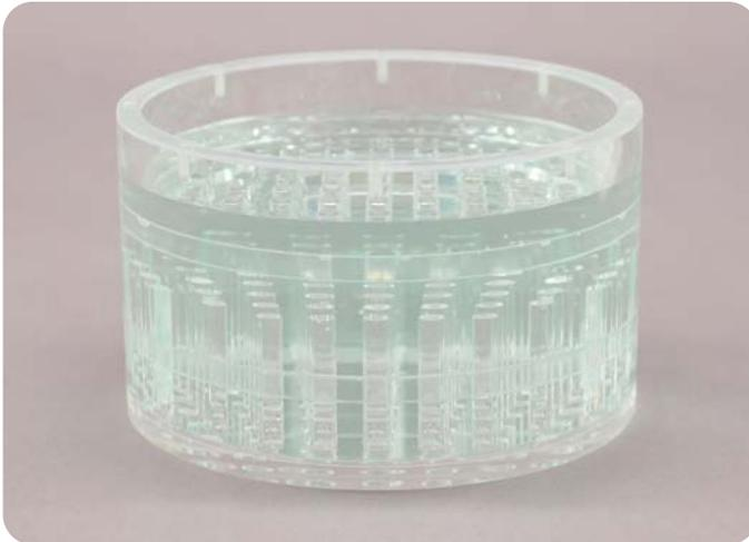
At this point, apply a small amount of jelly to the rubber portion between the lid and the main body of the phantom.
