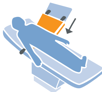
2). The cassette is inserted into the RadSlide and locked in place with hook-and-loop fasteners.
