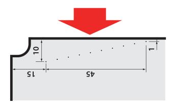
Depth range of 1-10 mm depth (10 targets are embedded)
