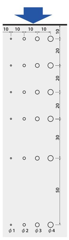
Target diameters 1, 2, 3, 4mm
