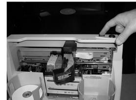
4. Open the ink carrier (purple cover for color on right side; gray for black on left side) by pressing on the blue lever, and if applicable, remove the existing ink cartridge from the carrier.
