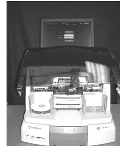
3. With the cover open, press the ink cartridge button to move the ink cartridge carrier to the load position.
