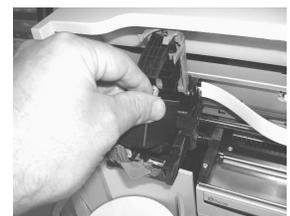
Note: 84-series and 101-series Recorders have only one ink carrier, which uses color ink only. On these models, the ink carrier cover and lever is black.
